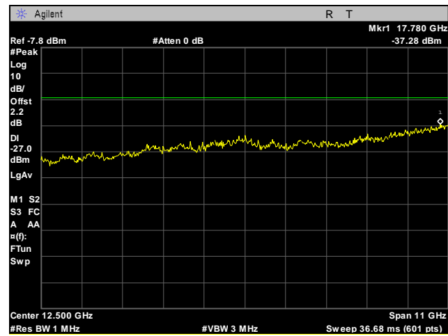
Plot 20. Radiated Spurious Emissions, 802.11a, Worst Case, 7 GHz – 18 GHz
