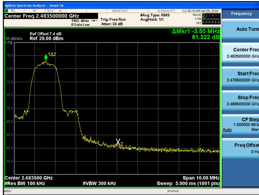
Test Plots with hopping (GFSK)
