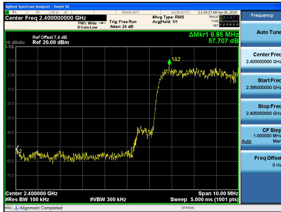
Test Plots with hopping (8DPSK)
