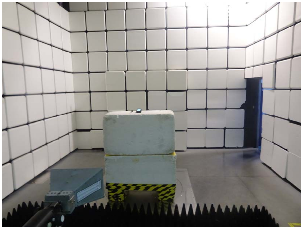
Picture 1: Radiated Spurious Emissions Test setup
