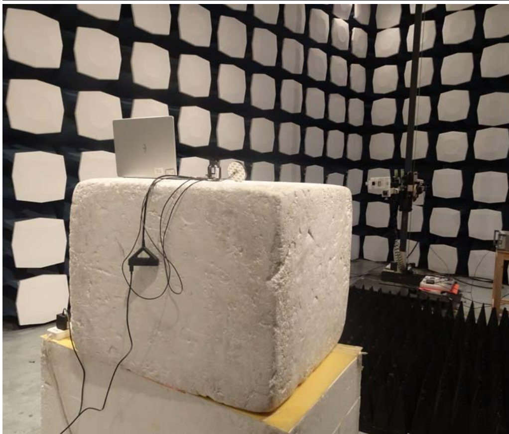
Picture 1 Radiated Emission Test Setup
