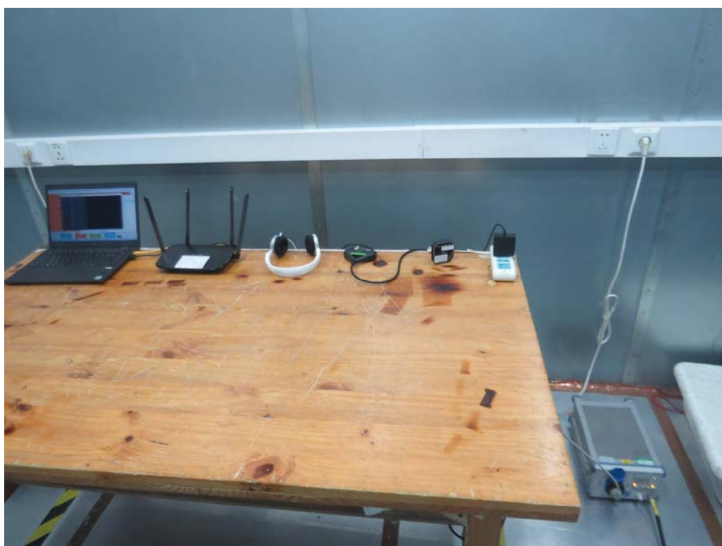
Picture 2: Conducted Emissions Test Setup
