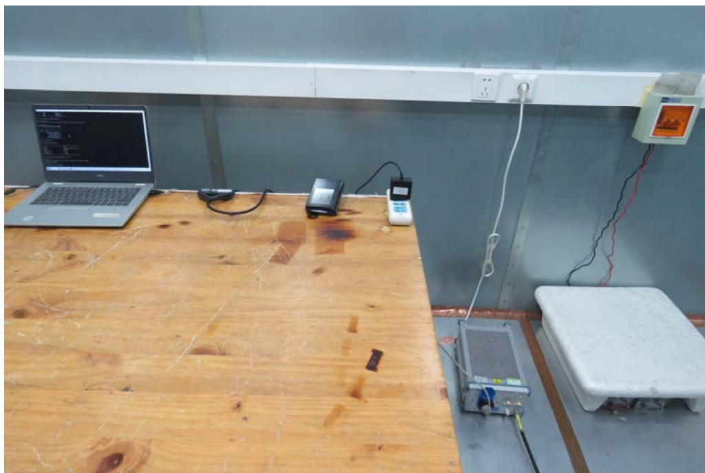
Picture 2 Conducted Emission Test Setup
