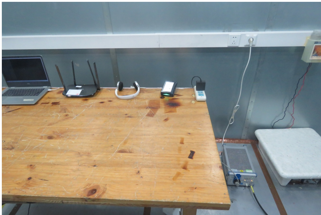
Picture 2: Conducted Emissions Test Setup
