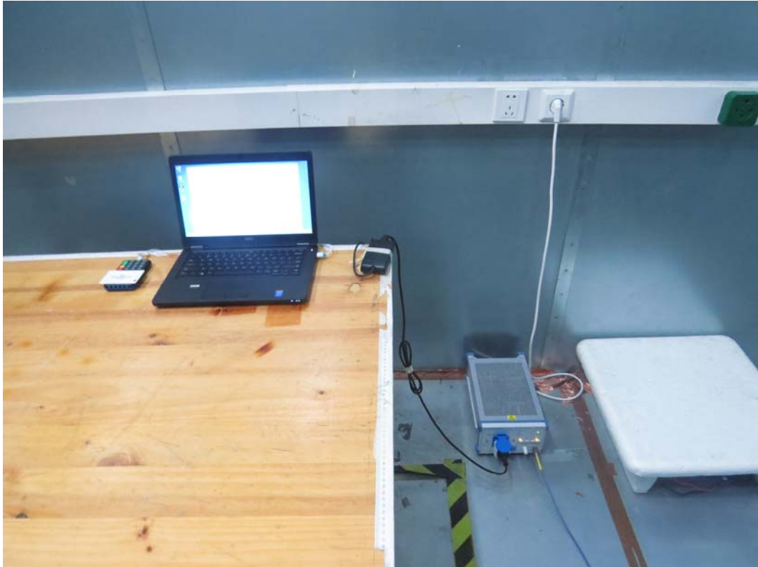
Picture 3 Conducted Emission Test Setup
