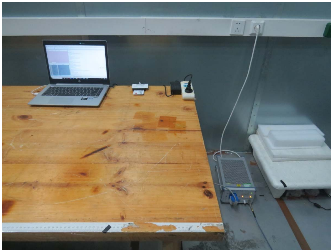
Picture 3 Conducted Emission Test Setup
