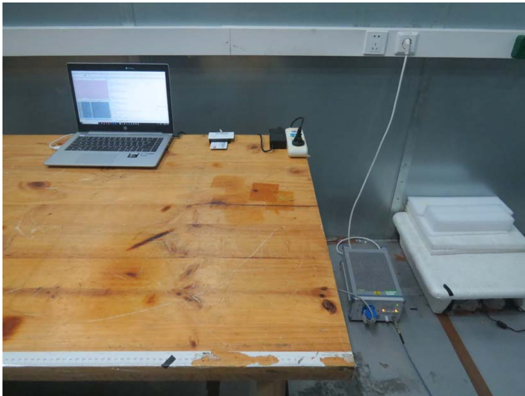
Picture 3 Conducted Emission Test Setup
