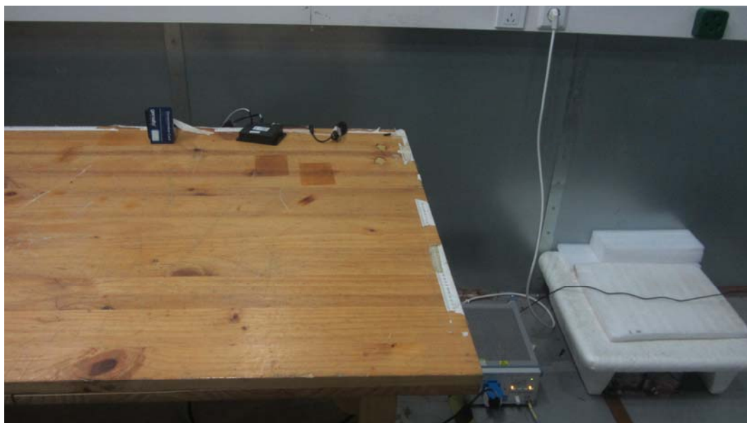
Picture 3 Conducted Emission Test Setup
