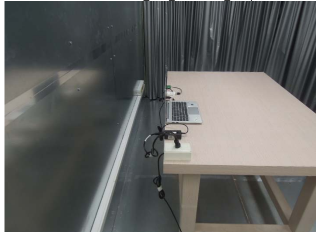
P15.225+RSS210 NFC Conduction Setup
