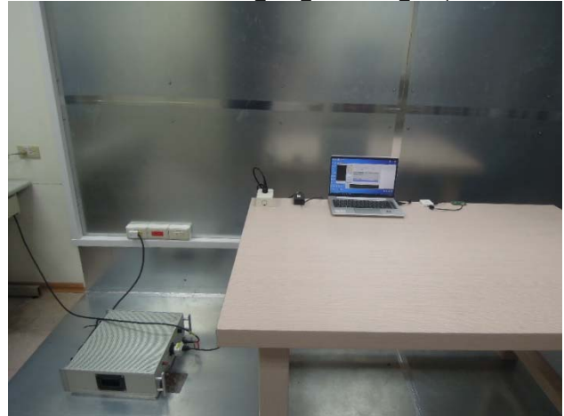
P15.225+RSS210 NFC Conduction Setup
