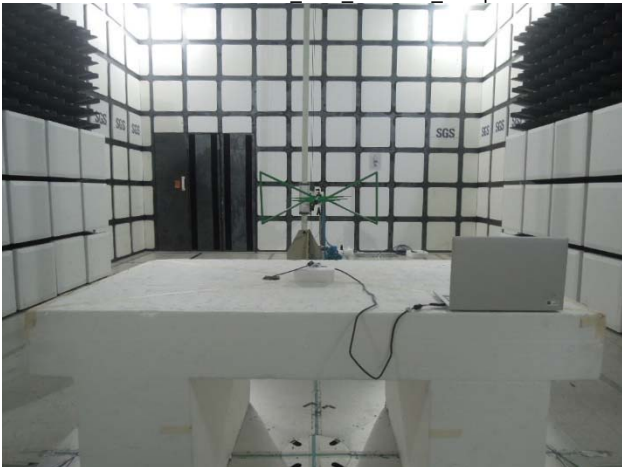
P15.225+RSS210 NFC Radiated Setup
