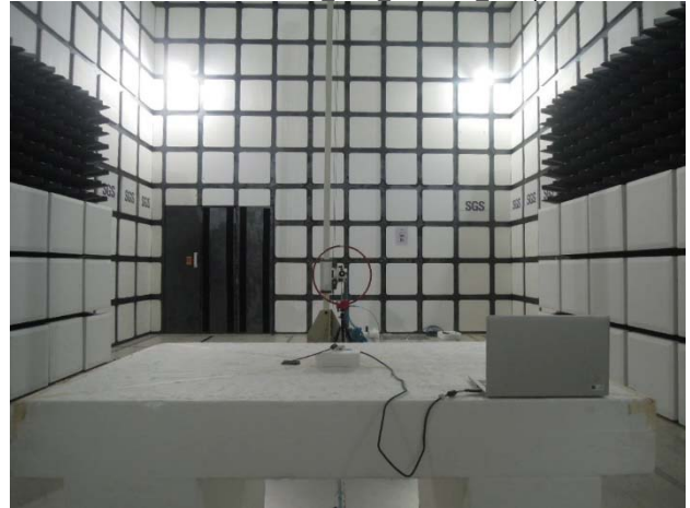
P15.225+RSS210 NFC Conduction Setup
