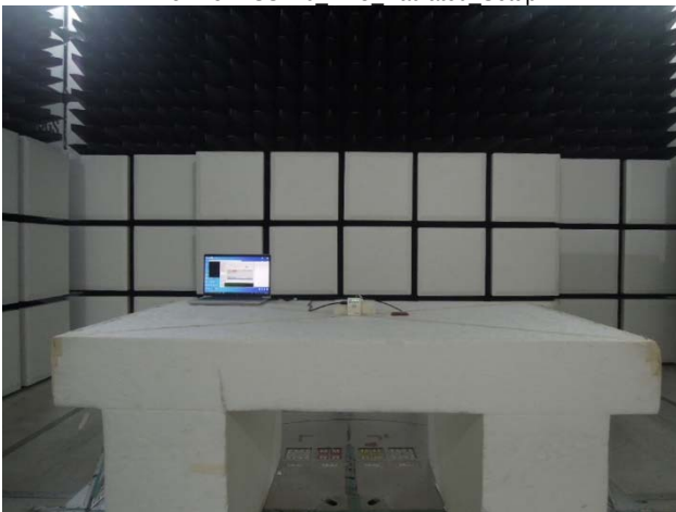
P15.225+RSS210 NFC Radiated Setup
