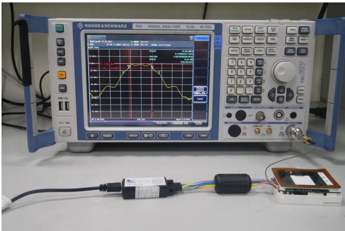
**RADIATED EMISSION SETUP PHOTOS****Below 1GHz**
