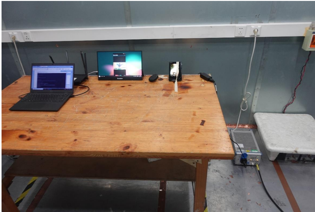
Picture 2: Conducted Emissions Test Setup
