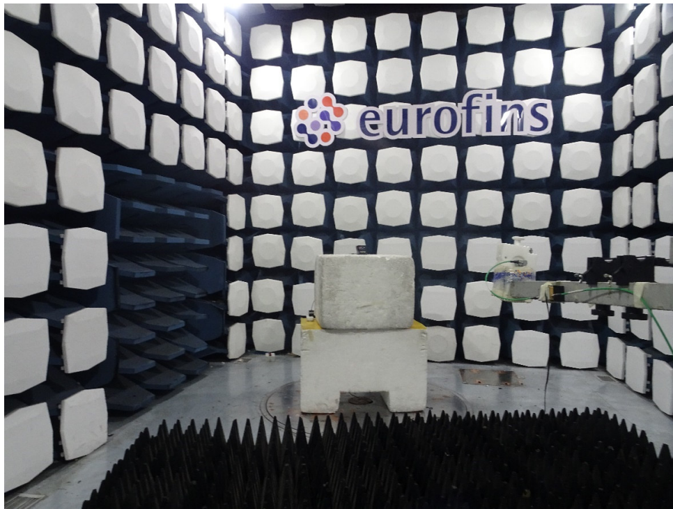
Picture 1 Radiated Emission Test Setup
