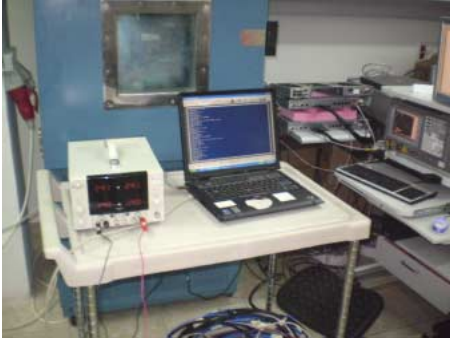
Photograph No.10 Frequency stability measurement setup
