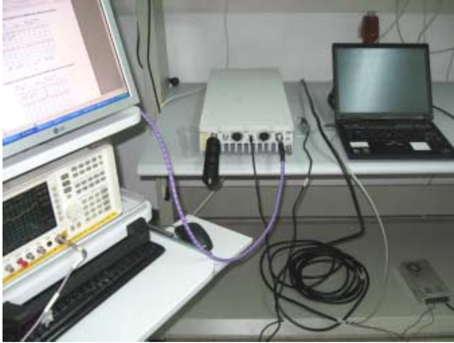
Photograph No.1 Peak output power, power spectral density, conducted spurious emissions measurement setup
