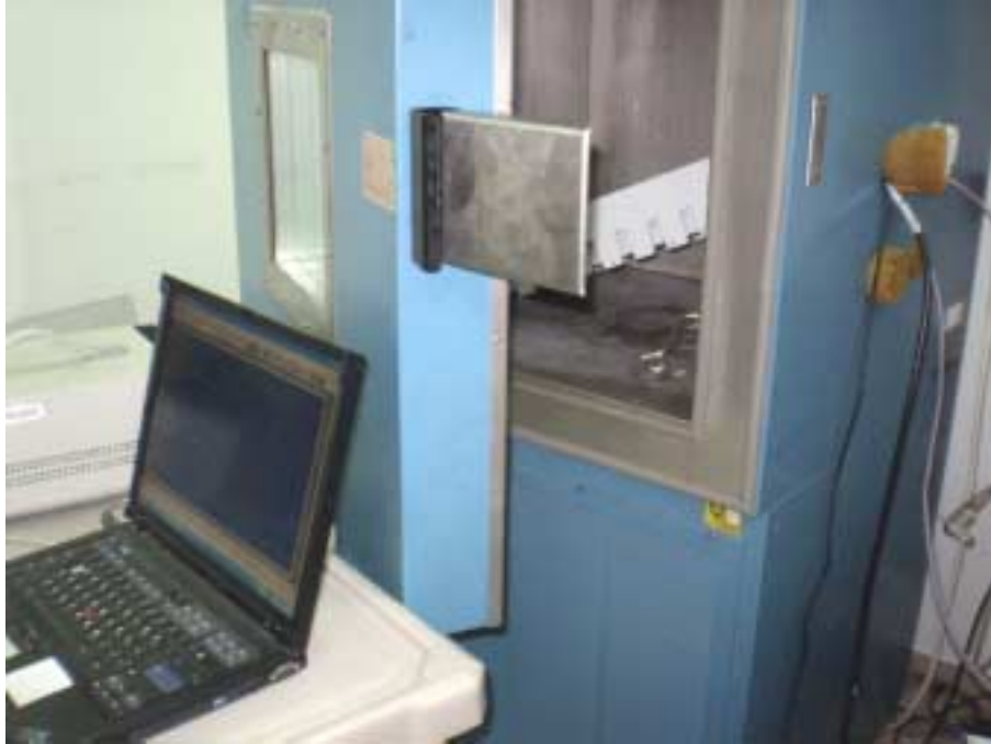
Photograph No.9 Frequency stability measurement setup
