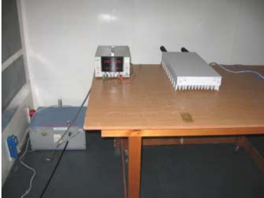
Photograph No.11 Conducted emissions measurement on AC line setup
