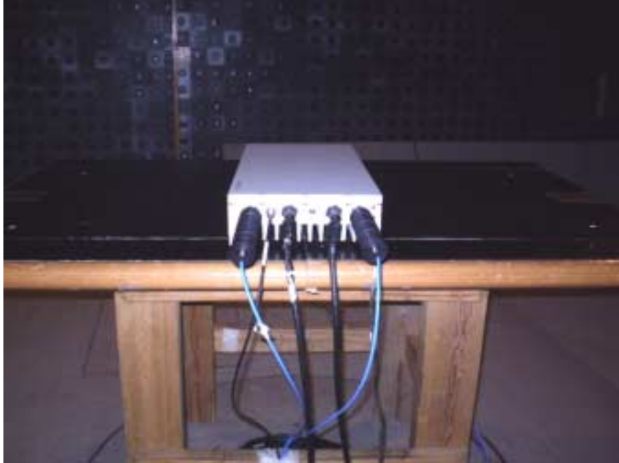
Photograph No.5 Radiated emissions measurement setup, EUT close view
