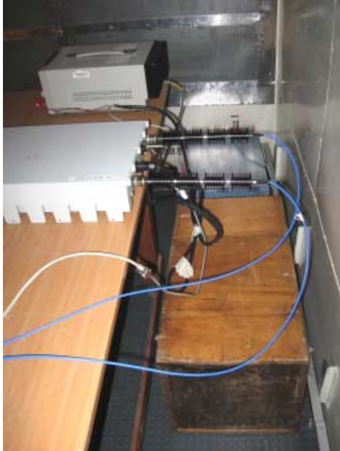
Photograph No.12 Conducted emissions measurement on AC line setup
