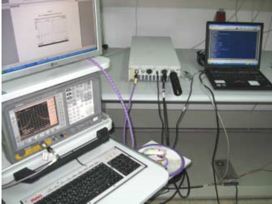
Photograph No.2 Occupied bandwidth and emission mask measurement setup
