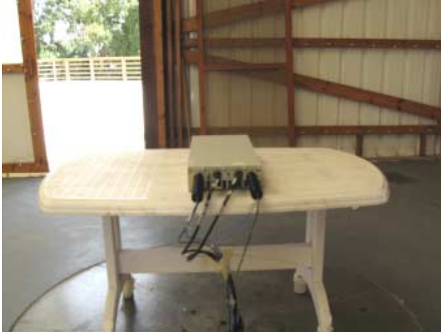
Photograph No.8 Radiated emissions measurement setup, EUT close view
