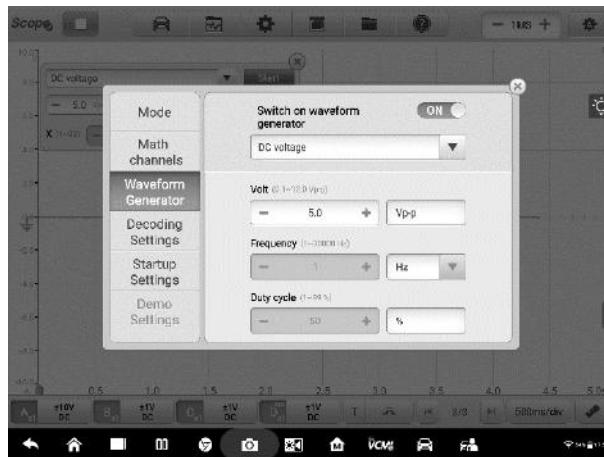
Figure 1-22 Sample Waveform generator Settings Screen
