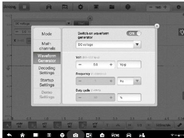
Figure 1-21 Sample Waveform Generator Setting Screen
