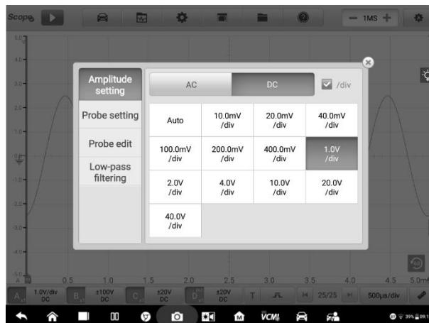
Figure 1-51 Sample Amplitude Setting Screen (DC 1.0V/div)
