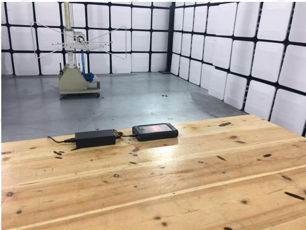
Photo of Radiation Emission Test
