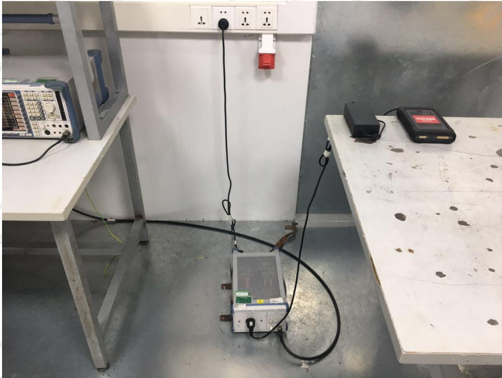
Photo of Conducted Emission Measurement
