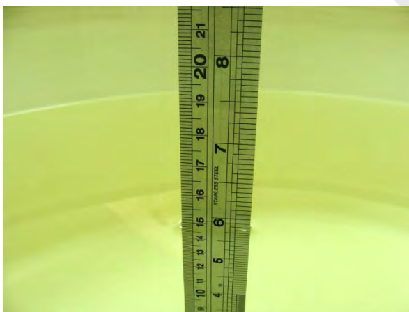
Photo of Liquid Height for Body SAR
