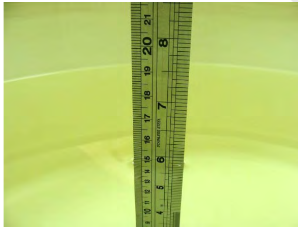
Photo of Liquid Height for Body SAR
