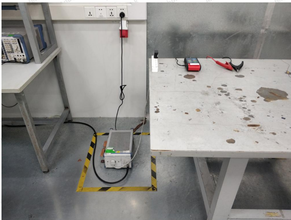
Photo of Conducted Emission Measurement
