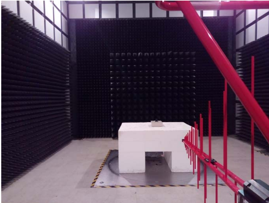
Radiated Emissions View (Below 1 GHz)
