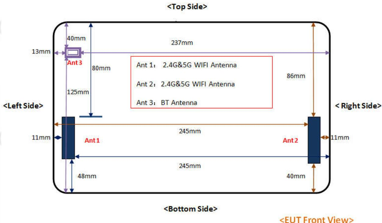
Note: 1) Per KDB 616217, because the diagonal Length is >200mm, it is considered a "tablet" device and need to test 0mm 1g Body SAR.
