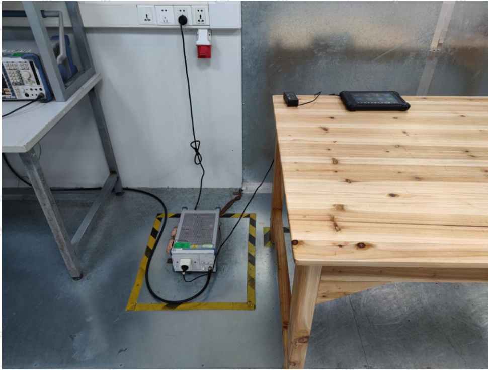
Photo of Conducted Emission Measurement
