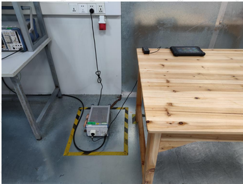
Photo of Conducted Emission Measurement
