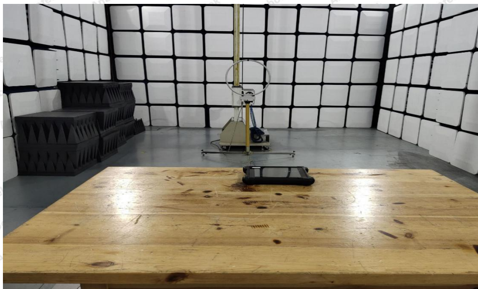
Photo of Radiation Emission Test
