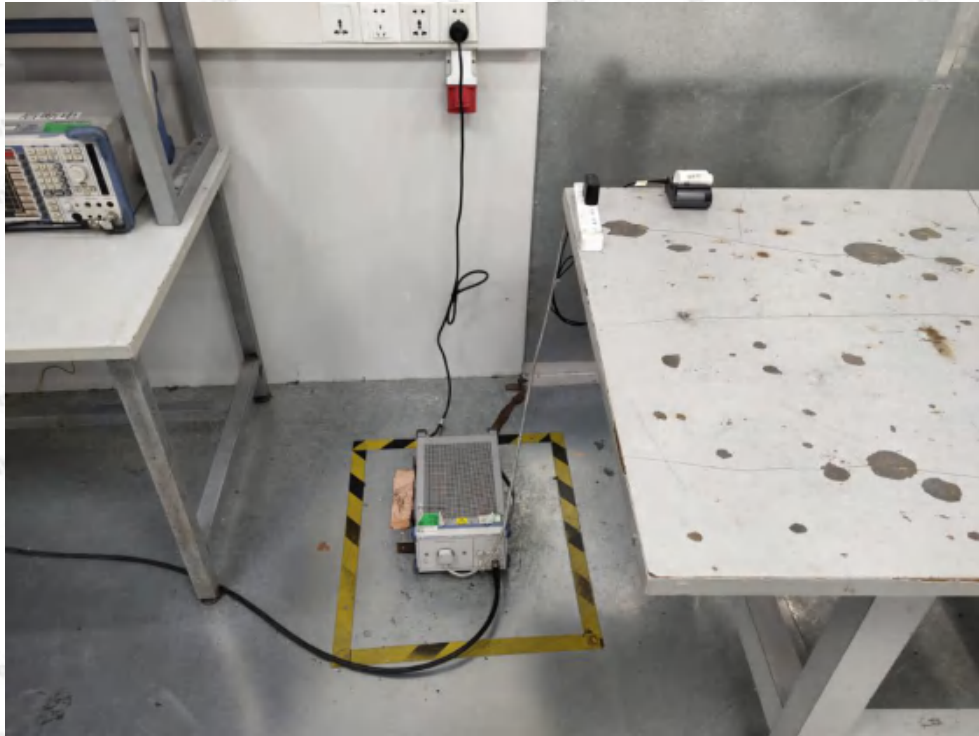
Photo of Power Line Conducted Emission Test
