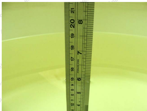
Photo of Liquid Height for Body SAR
