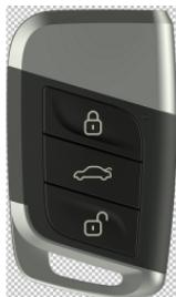
Unlock key: Unlock the vehicle,
