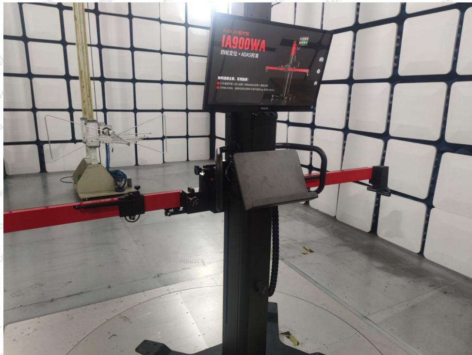
Photo of Radiation Emission Test
