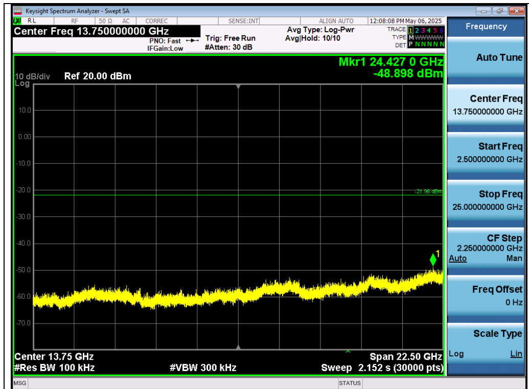
Test_Graph_LE1M_ANT1_2480_1Mbps_Higher Band Emissions
