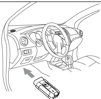
\*Choose an adapter (Deutsch-6, Deutsch-9, or PLC adapter) according to vehicle's DLC.
