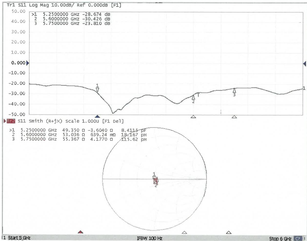
Impedance and Return Loss Test-Head (2025.02.11)
