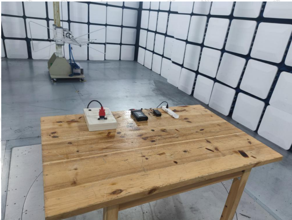
Photo of Radiation Emission Test
