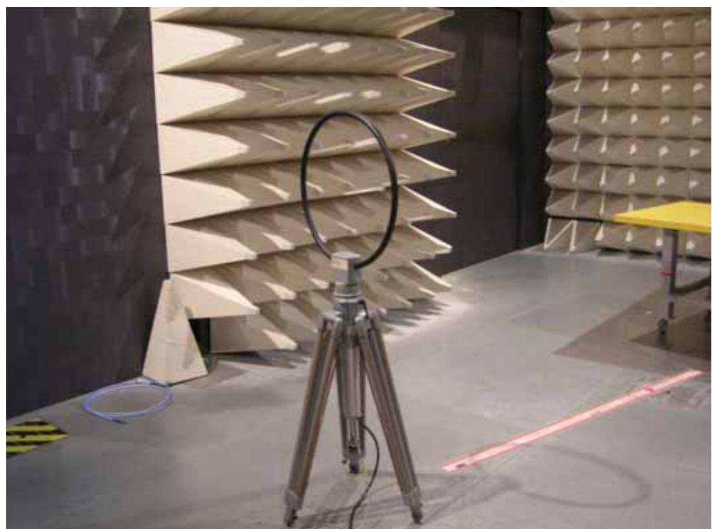
For radiated emissions 30MHz~1GHz
