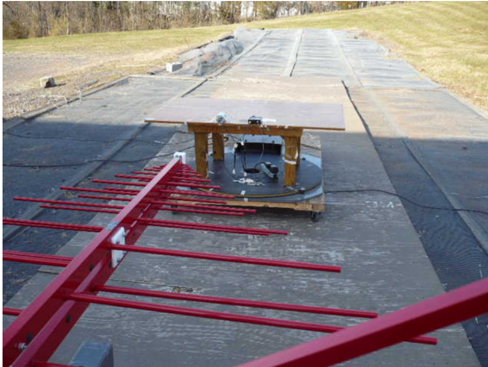
Biconilog Antenna, Horizontal Polarization, 30 to 1000 MHz
