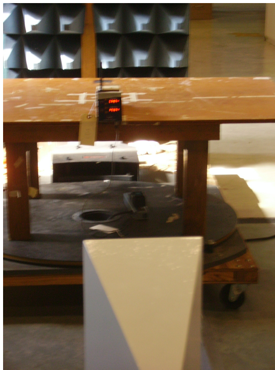
High Gain Horn, Horizontal Polarization, 8.2 to 12.4 GHz
