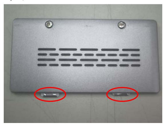
below hull use conduct electricity cloth and RAM door connect and conduct electricity fluent.
