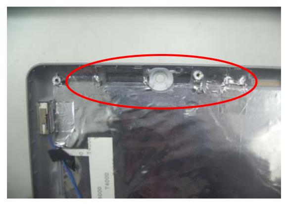
the panel post top gasket must with A case the aluminum foil conduct electricity fluent.
