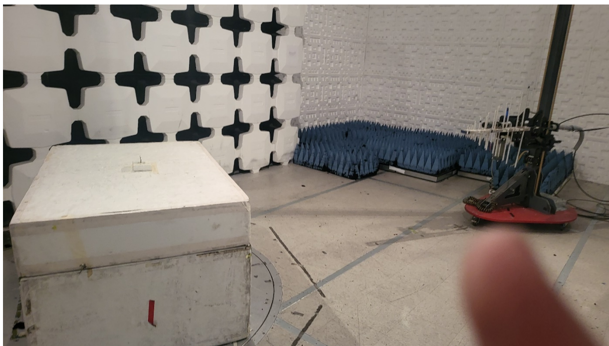
Figure 4. Test Configuration 200- 1000 MHz using Log Periodic Antenna
