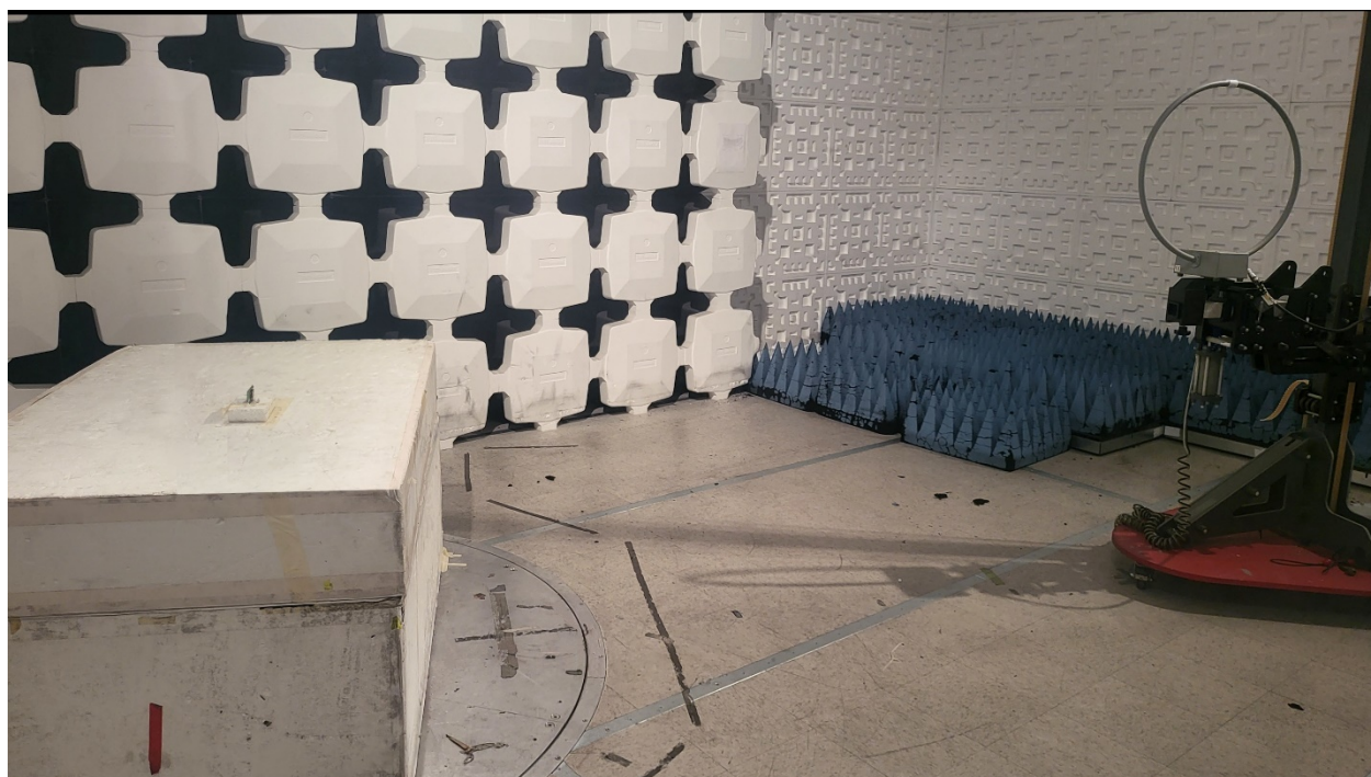
Figure 2. Test Configuration below 30 MHz using Loop Antenna
