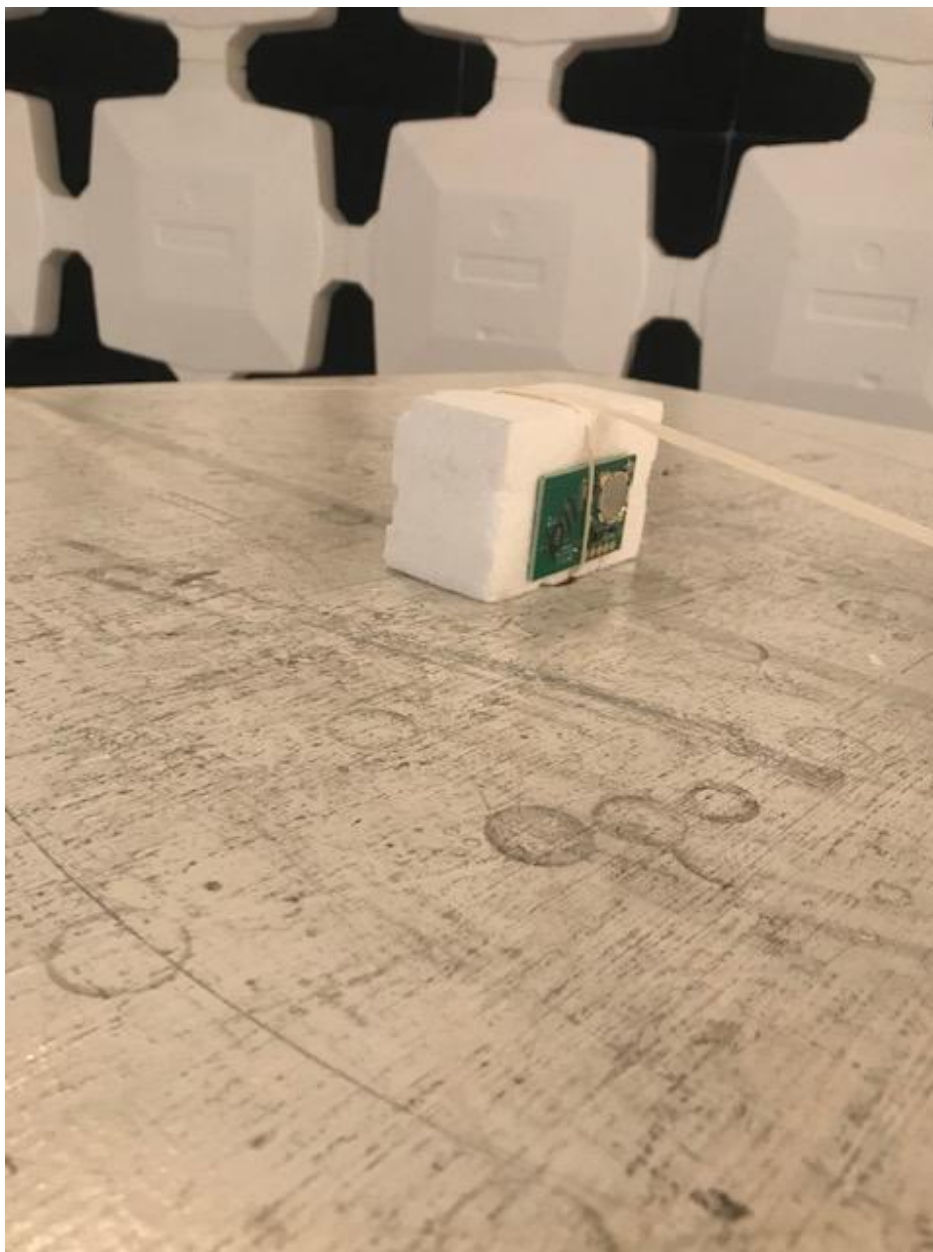
Figure 1. Radiated Emissions Test Setup
