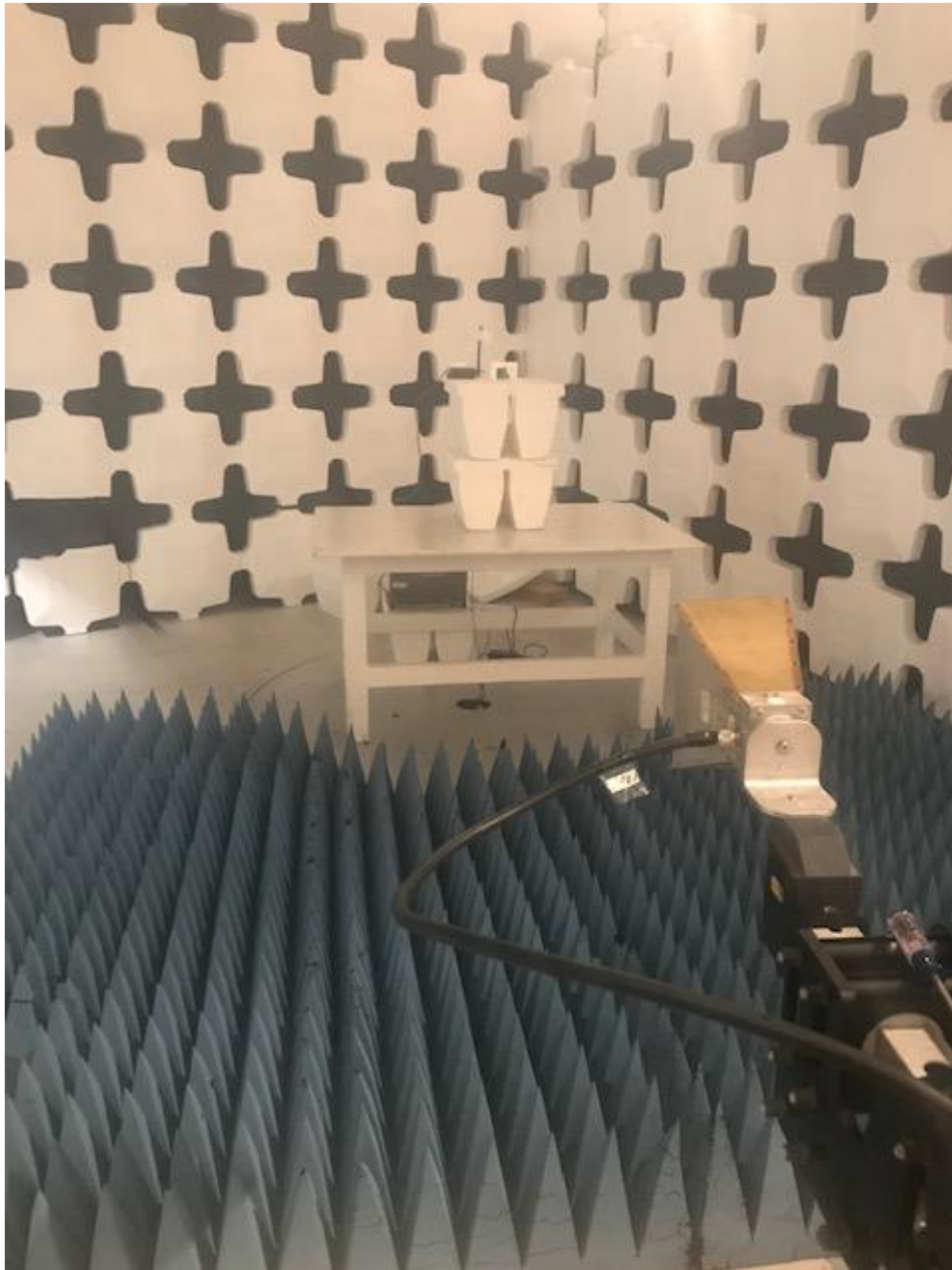
Figure 6. Radiated Emissions Test Setup (Above 1, Intentional Emissions)
