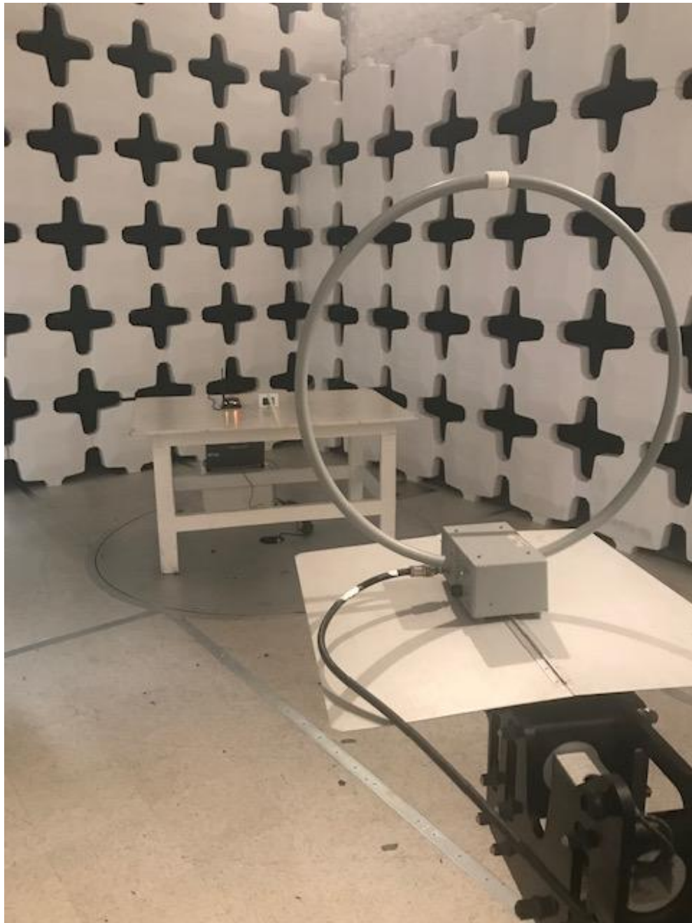
Figure 2. Radiated Emissions Test Setup (9 kHz - 30 MHz)
