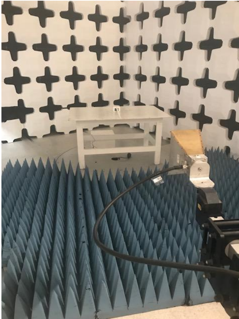
Figure 5. Radiated Emissions Test Setup (Above 1 GHz, Unintentional Emissions)
