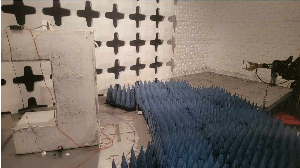
Figure 8. Test Configuration above 1 GHz using Horn Antenna Intentional Emissions
