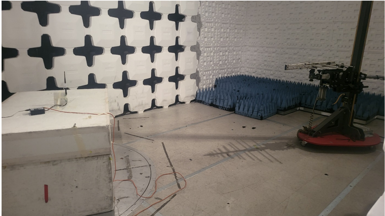
Figure 6. Test Configuration 200- 1000 MHz using Log Periodic Antenna Intentional Emissions
