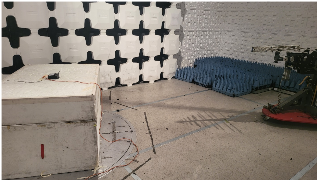
Figure 7. Test Configuration 200- 1000 MHz using Log Periodic Antenna Unintentional Emissions (including co-location evaluation)
