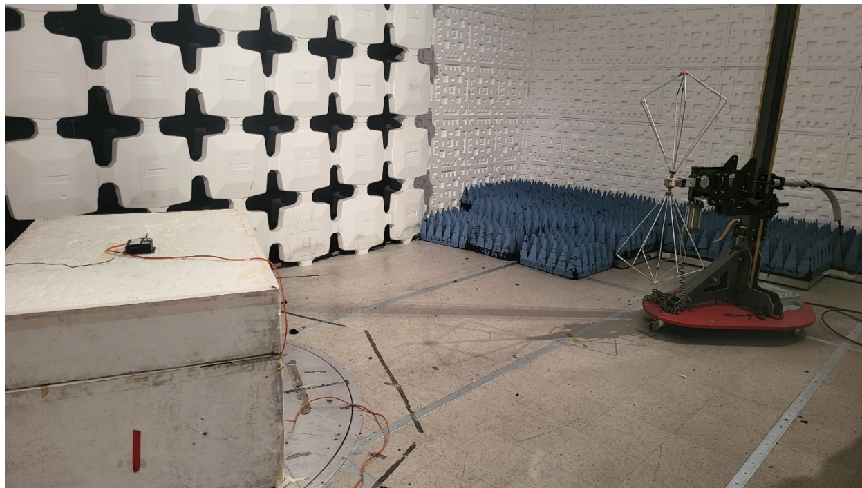
Figure 5. Test Configuration 30-200 MHz using Biconical Antenna Unintentional Emissions (including co-location evaluation)
