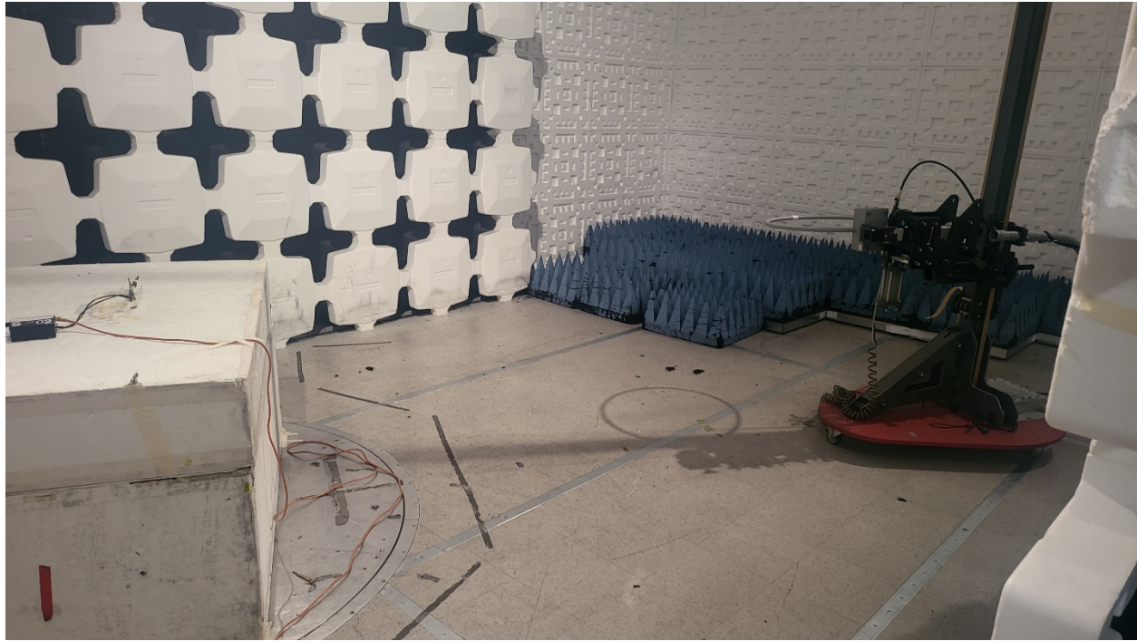
Figure 3. Test Configuration below 30 MHz using Loop Antenna
