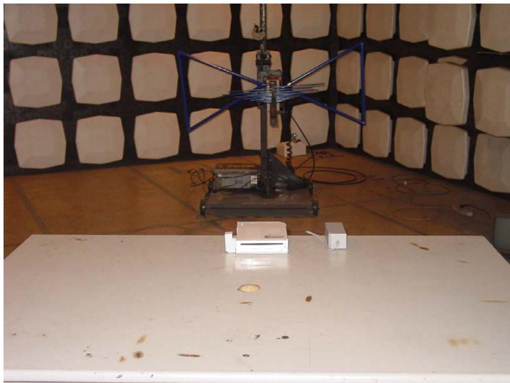
Set-up for radiated measurements (above 1G)
