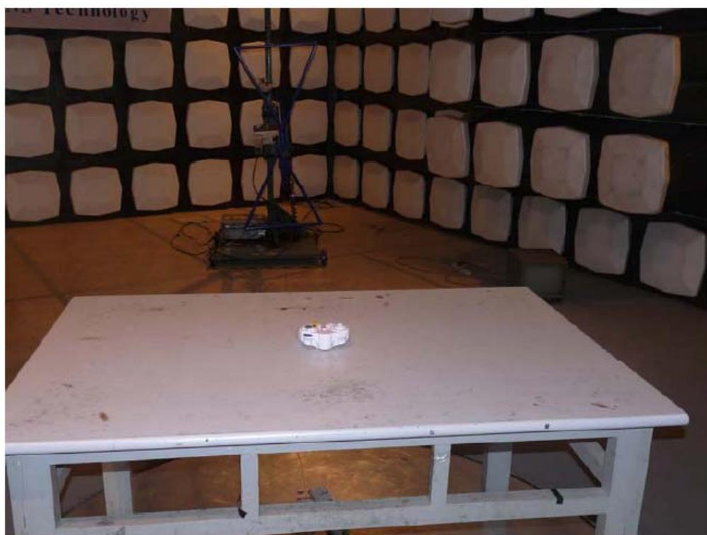
Set-up for radiated measurements (above 1G)
