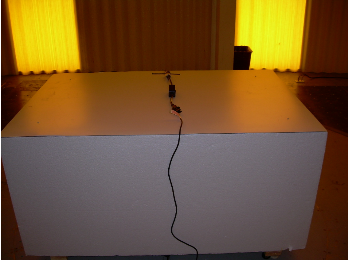
View of the Radiated Emission Test Setup (Horizontal Face Alignment)
