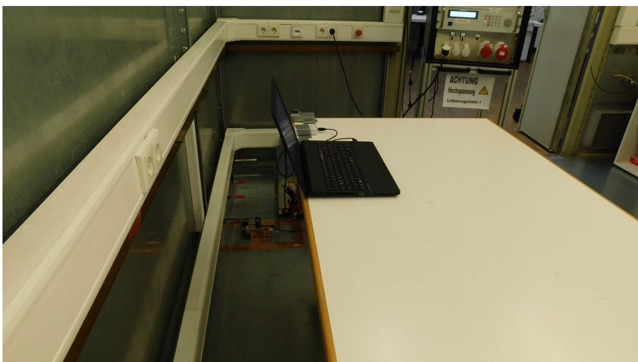
Picture 6: Test setup AC power line conducted emissions (rear view)
