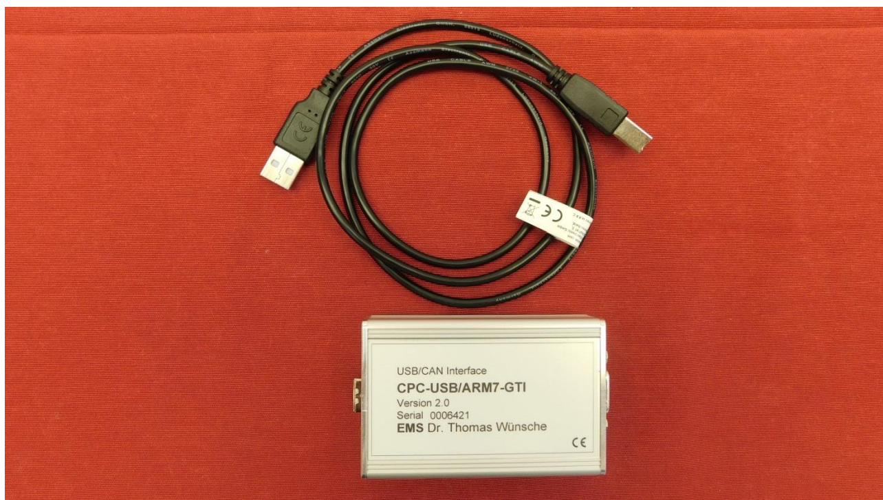
Picture 13: CAN interface with USB cable
