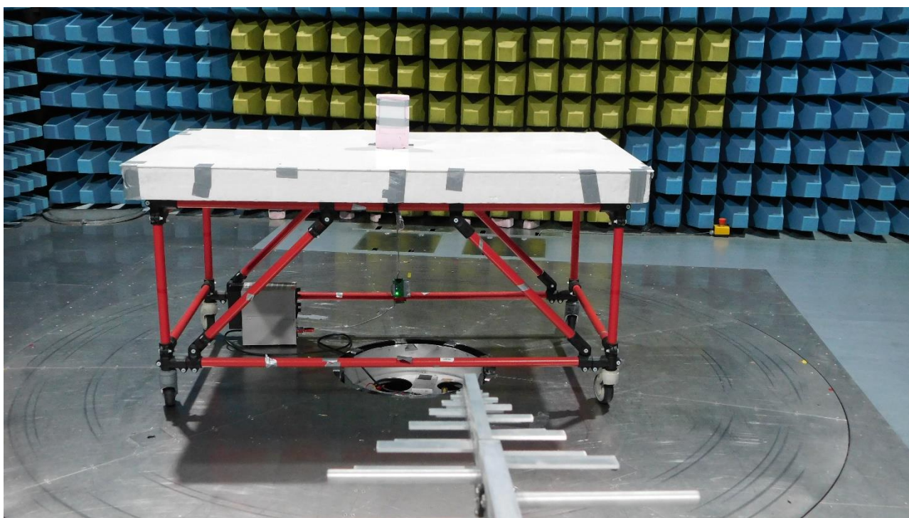
Picture 21: SAC, radiated emission test 30 MHz - 1 GHz (rear view)
