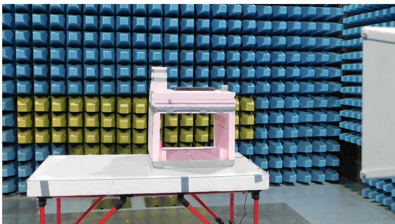
Picture 6: SAC, radiated emission test 1 GHz – 17 GHz (rear view)
