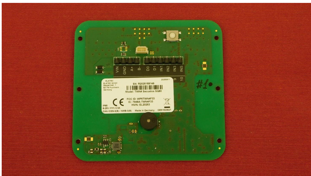
Picture 2: Opened EUT – bottom view
