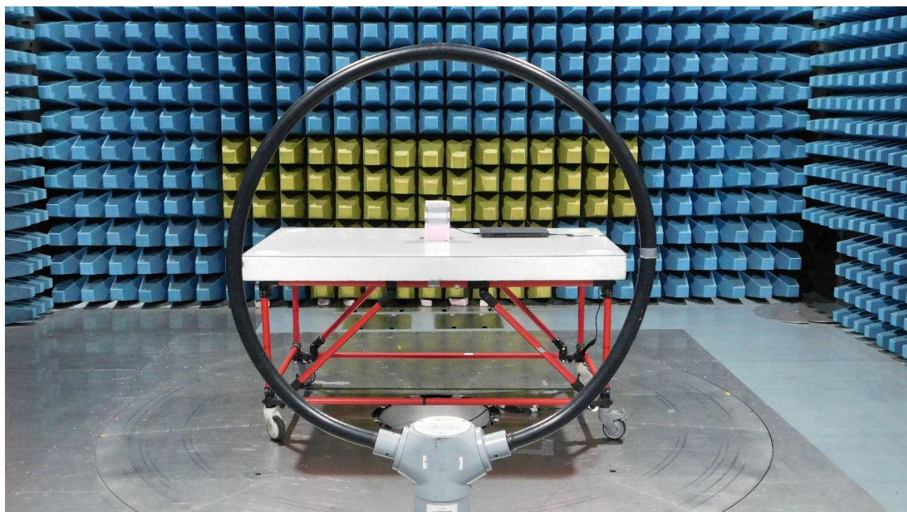
Picture 2: SAC, test setup radiated emission test 9 kHz - 30 MHz (rear view)
