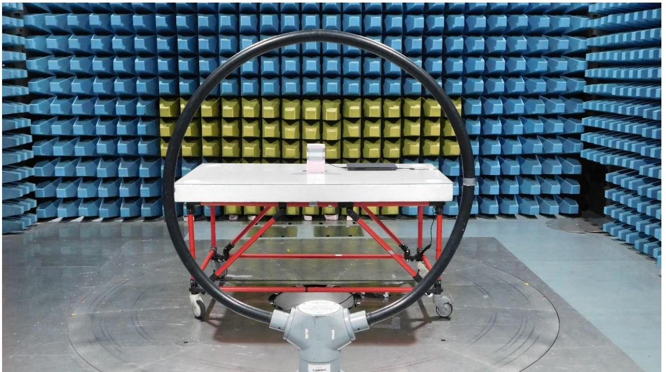
Picture 2: SAC, test setup radiated emission test 9 kHz - 30 MHz (rear view)
