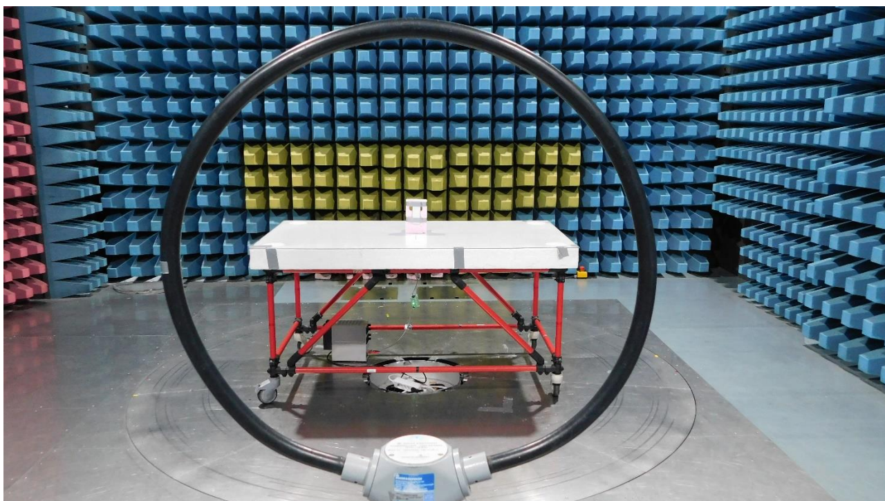
Picture 17: SAC, test setup radiated emission test 9 kHz - 30 MHz (rear view)
