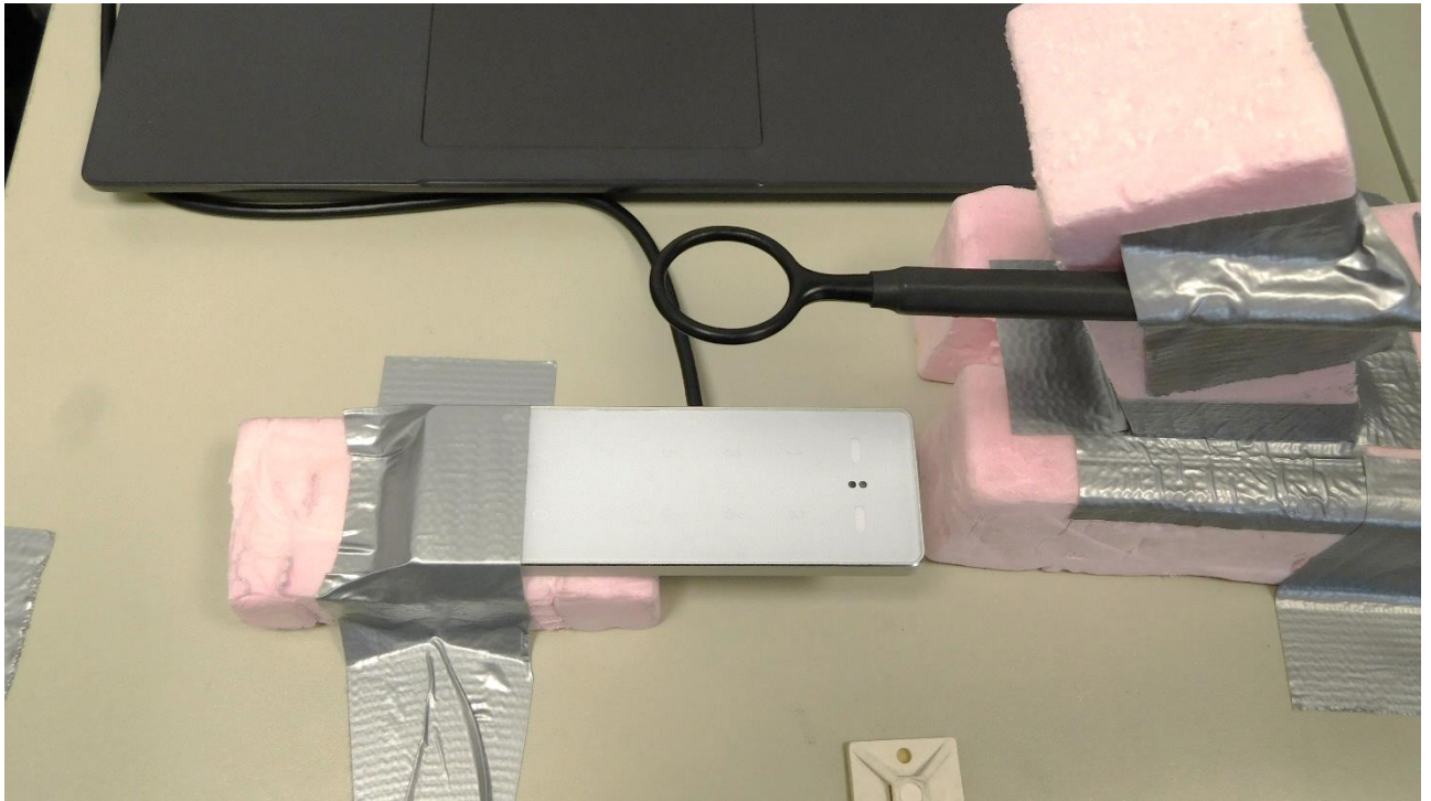
Picture 9: Test setup for occupied bandwidth tests
