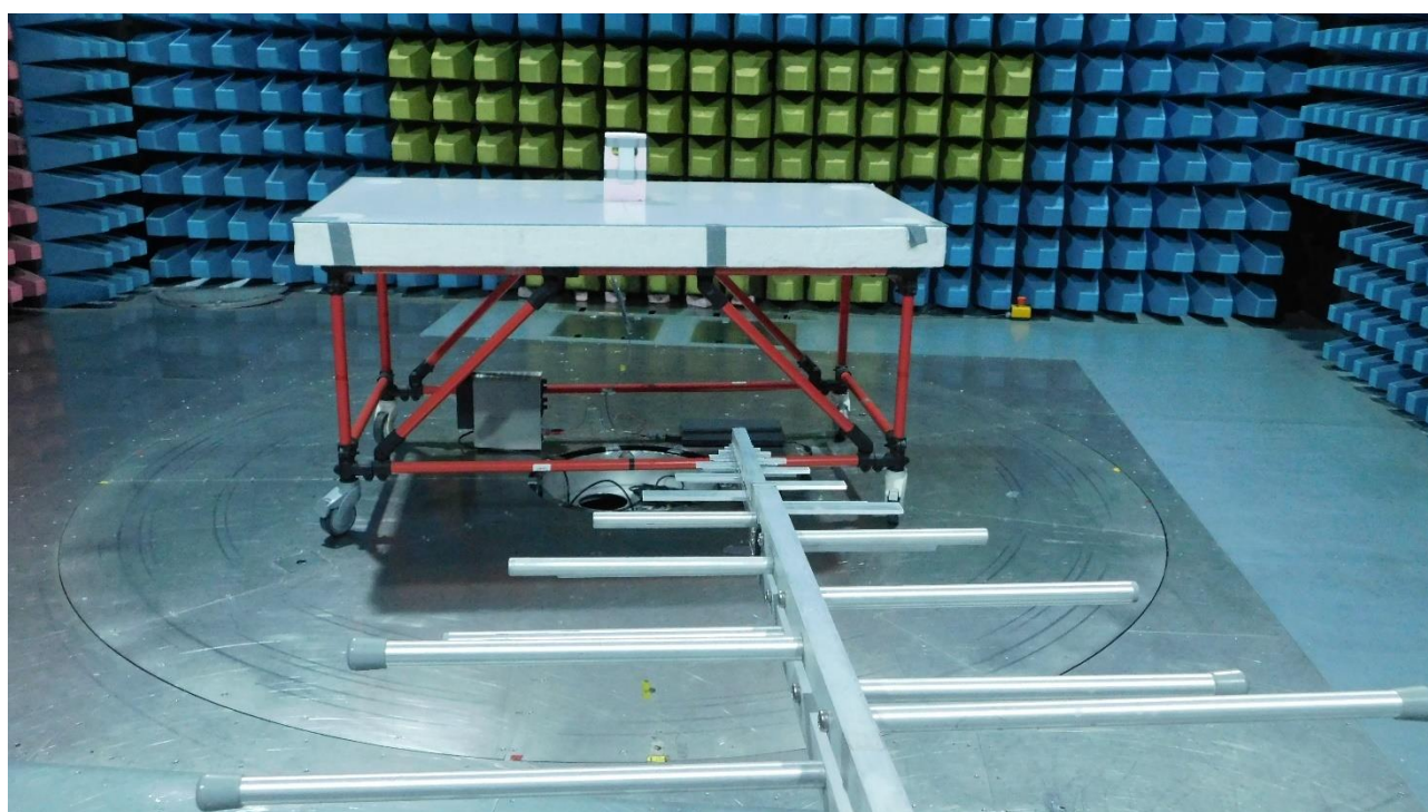
Picture 13: SAC, radiated emission test 30 MHz - 1 GHz (rear view)
