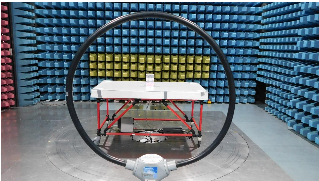
Picture 11: SAC, test setup radiated emission test 9 kHz - 30 MHz (rear view)
