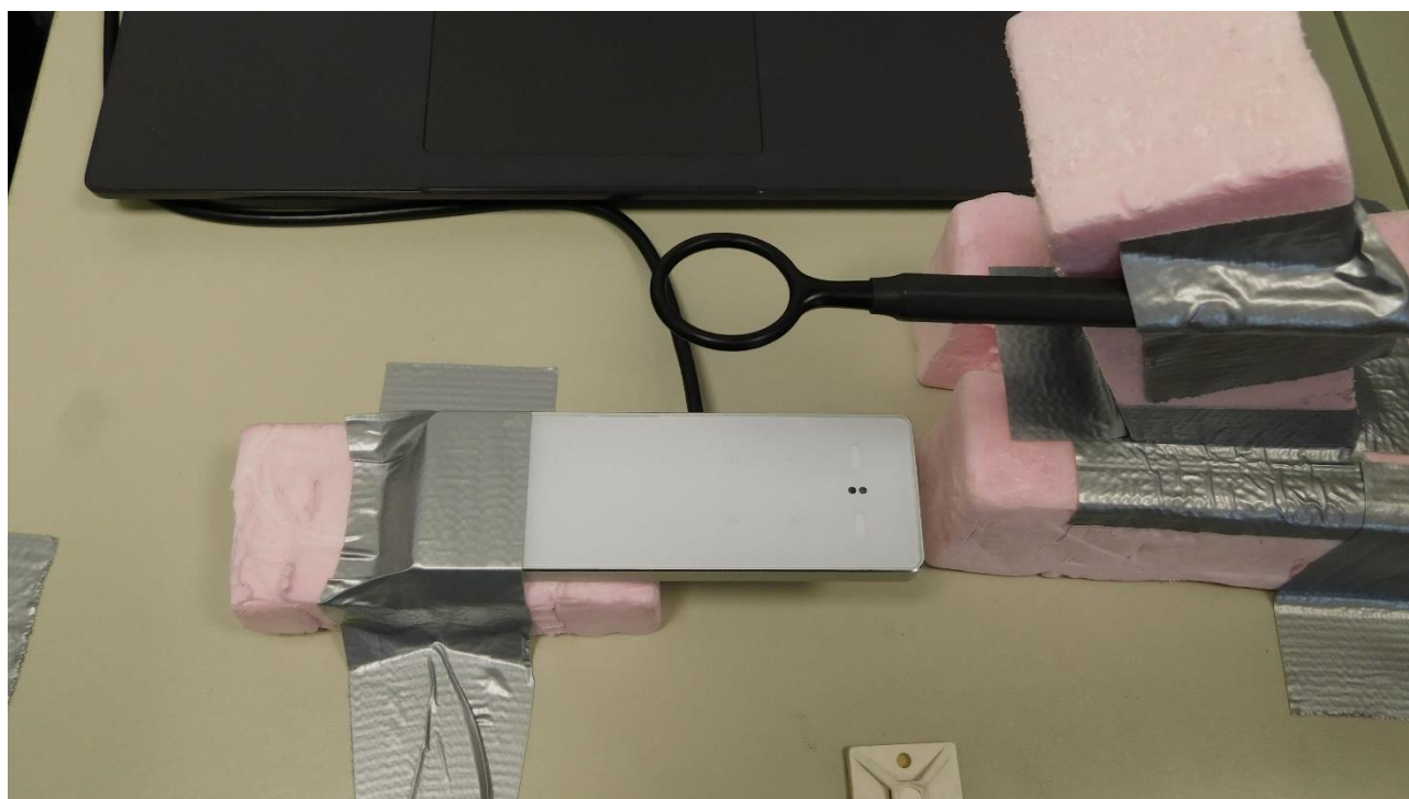
Picture 9: Test setup for occupied bandwidth tests
