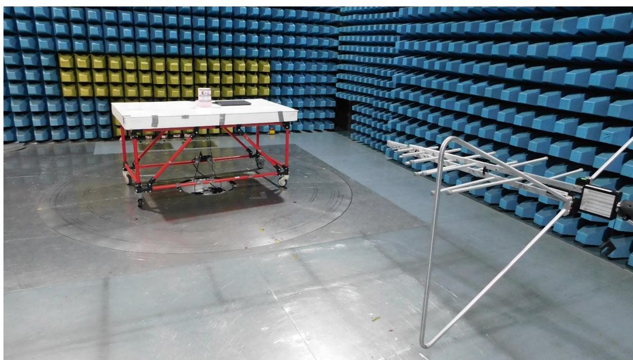
Picture 4: SAC, radiated emission test 30 MHz - 1 GHz (rear view)
