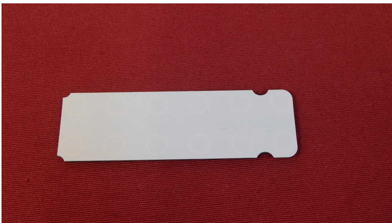
Picture 4: Touch PCB – top side
